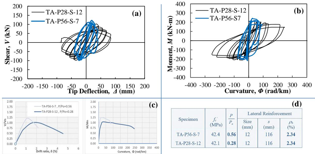
Figure 4. Effect of Axial Load Level: (a)  $V-\delta$  hysteresis response, (b)  $M-\phi$  hysteresis response, (c) envelope curves, and (d) specimen details
