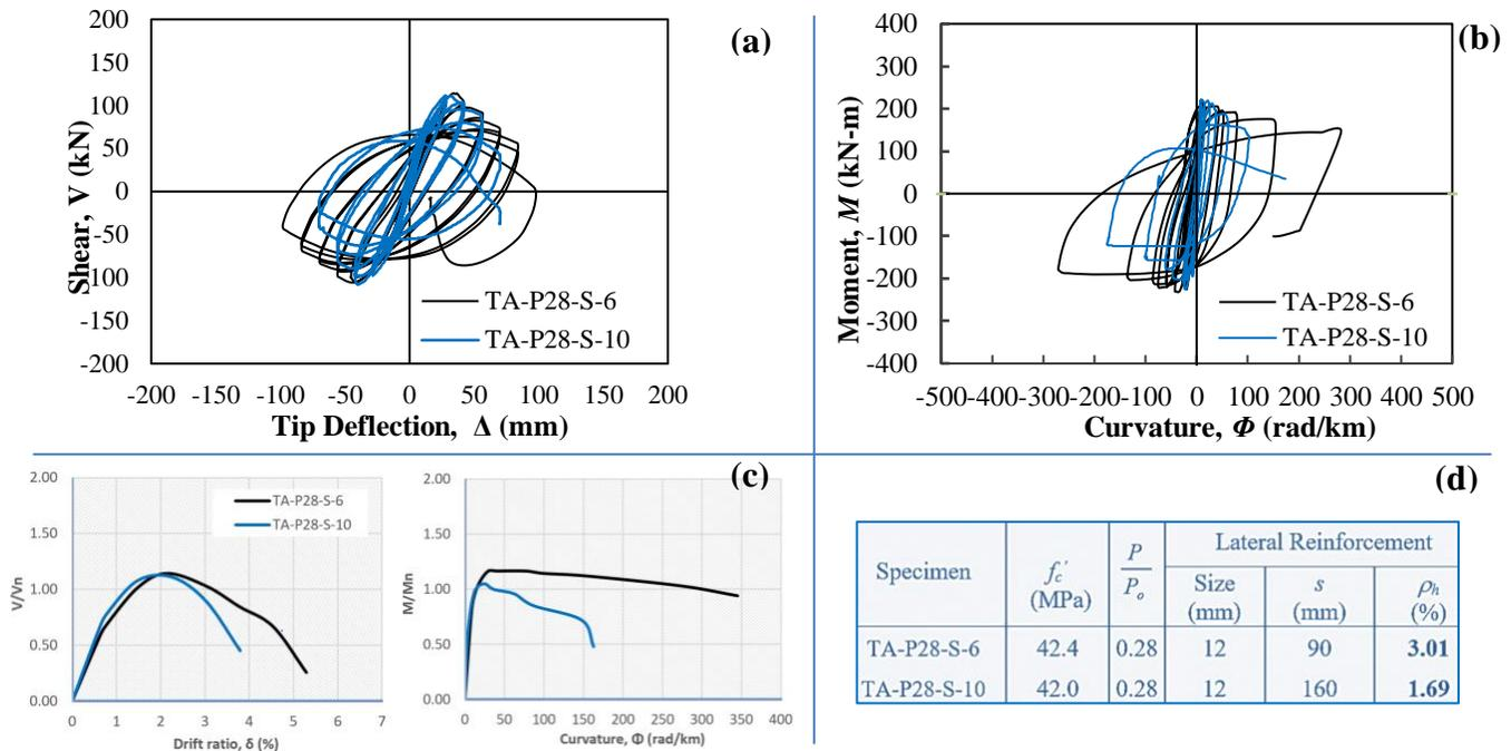
Figure 5. Effect of amount of lateral reinforcement: (a)  $V-\delta$  hysteresis response, (b)  $M-\phi$  hysteresis response, (c) envelope curves, and (d) specimen details
