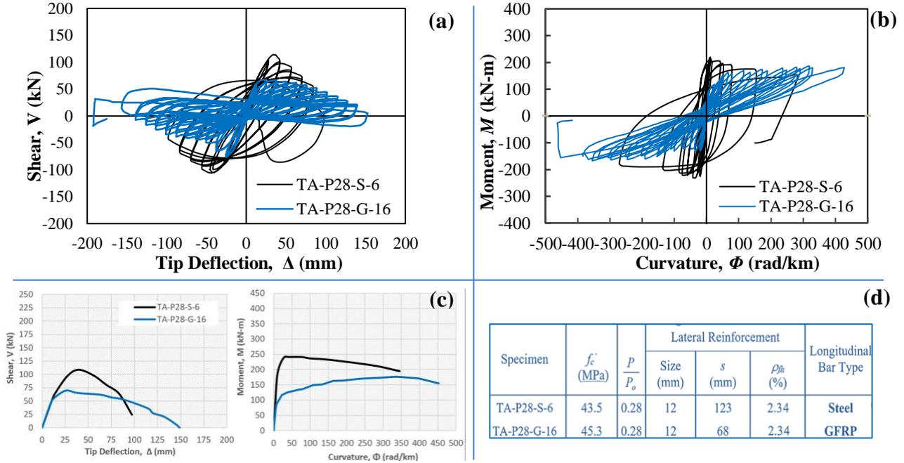
Figure 7. Effect of Longitudinal Bar Type: (a)  $V-\delta$  hysteresis response, (b)  $M-\phi$  hysteresis response, (c) envelope curves, and (d) specimen details
