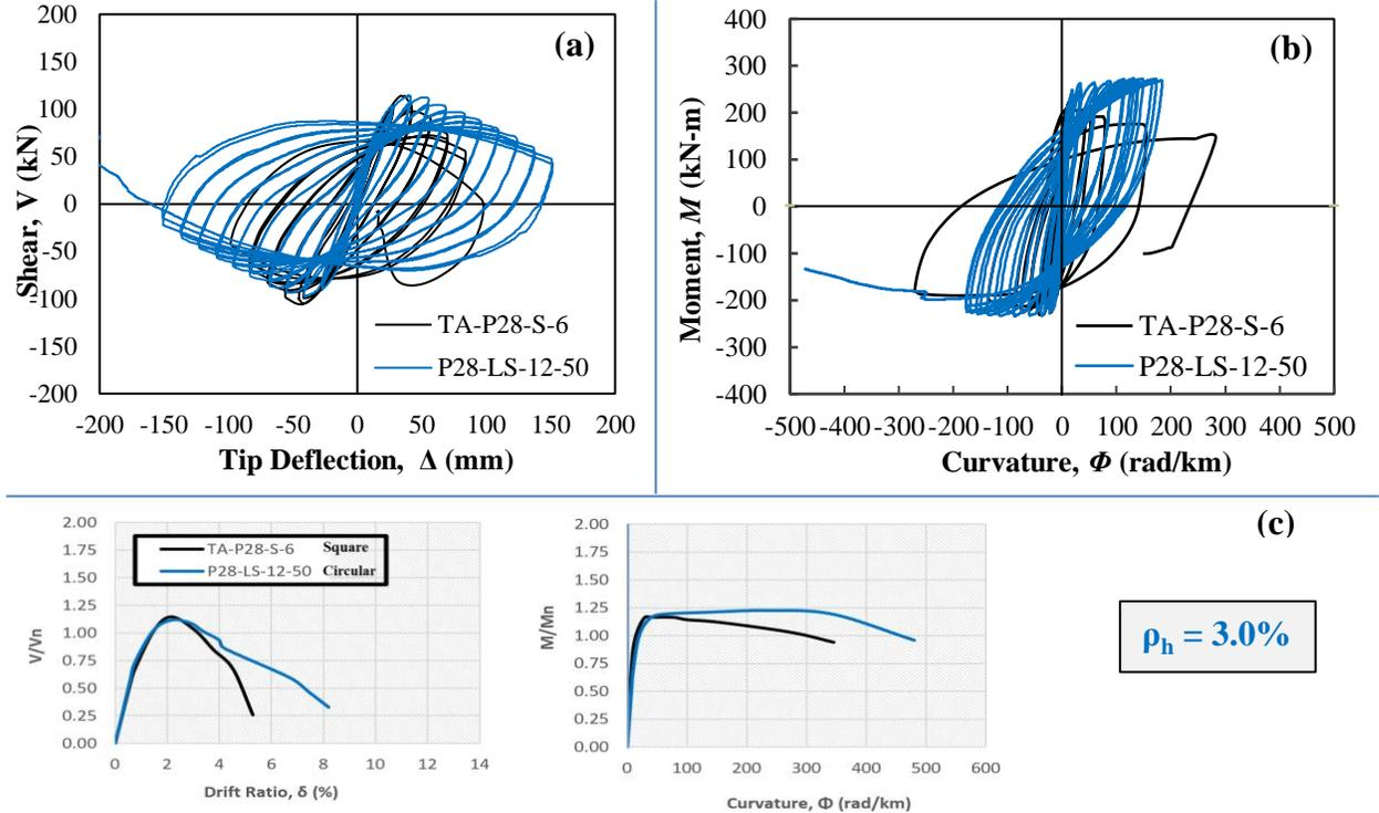
Figure 9. Effect of Section Geometry: (a)  $V-\delta$  hysteresis response, (b)  $M-\phi$  hysteresis response, and (c) envelope curves
